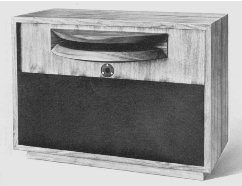
Figure 11.5. Classic dual-380 mm two-way studio monitor configuration with wide-angle diffraction high-frequency horn. This particular 1970s embodiment also added a 25 mm exit compression driver without a horn for ultra-high-frequency augmentation. (Courtesy Westlake Audio.)
