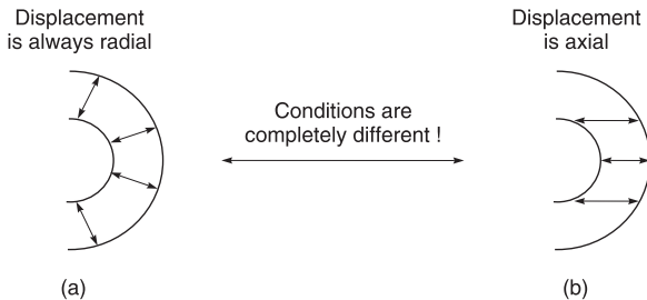
Figure 2.36. The myth of the dome. At (a) an ideal radiator would be a pulsating sphere. Dome at (b) resembles a sphere, but it does not pulsate; it moves in one axis and the results are quite different.
