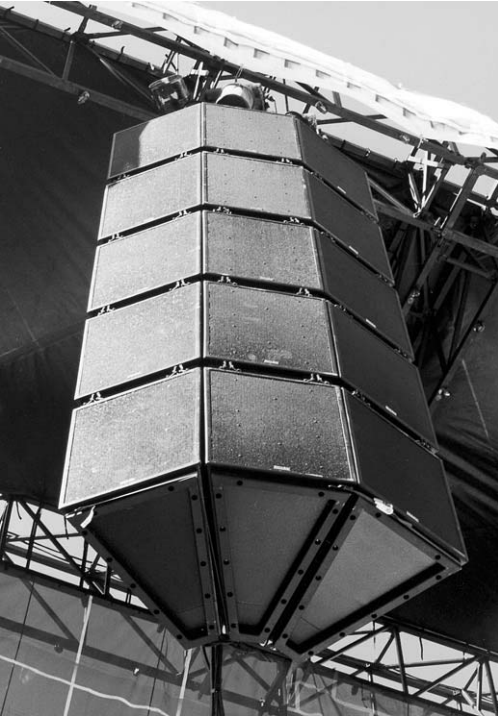
Figure 10.13. DSP-controlled loudspeaker array (Courtesy EAW).
